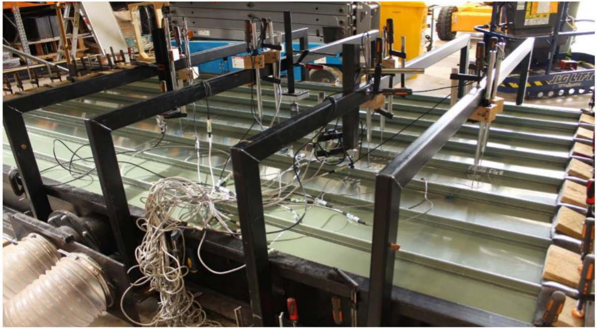
(a) Super seam claddings with pan width of 200 mm
