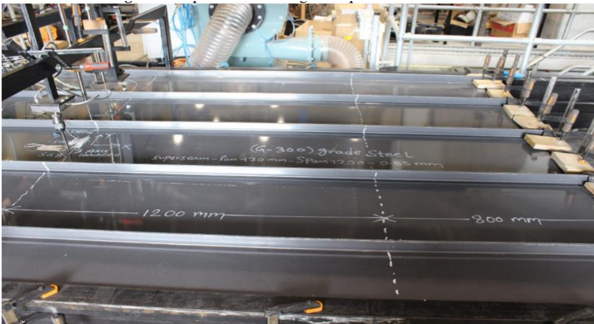
(b) Super seam claddings with pan width of 450 mm
